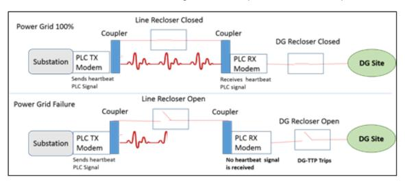
The DG-TTP Anti-Islanding Transfer Trip Protection Concept
